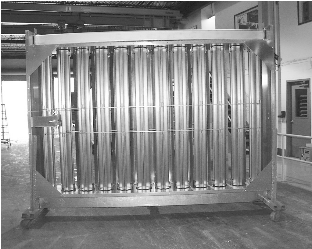
Photo of Direct-Coupled VIFB (Entering Air Side)
